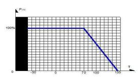
board (thermal resistance). The rated dissipation applies only if the permitted film temperature is not exceeded. These resistors do not feature a limited lifetime when operated within the permissible limits. However, resistance value drift increasing over operating time may result in exceeding a limit acceptable to the specific application, thereby establishing a functional lifetime.
